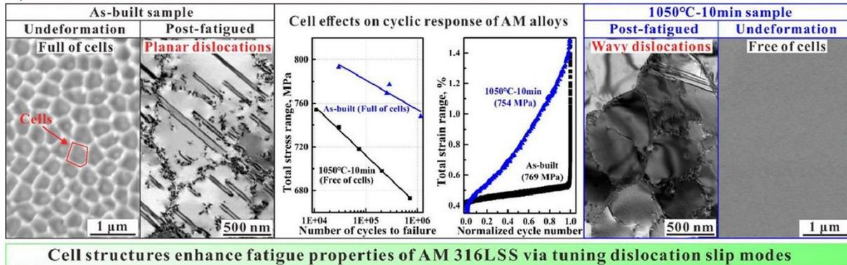
**Cell structures enhance fatigue properties of AM 316LSS via tuning dislocation slip modes**
