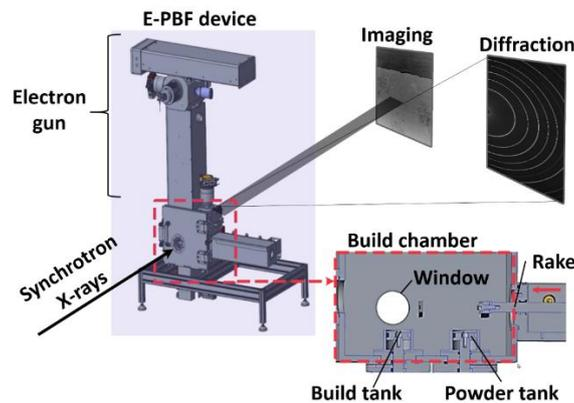
Powder bed fusion (PBF) technologies are successfully implemented processes in additive manufacturing (AM) of metal components. While Laser-PBF (L-PBF) has a larger share of production capacities, Electron beam-PBF (E-PBF) is particularly promising for manufacturing of high-performance alloys that need to be processed at high temperatures and under vacuum.
